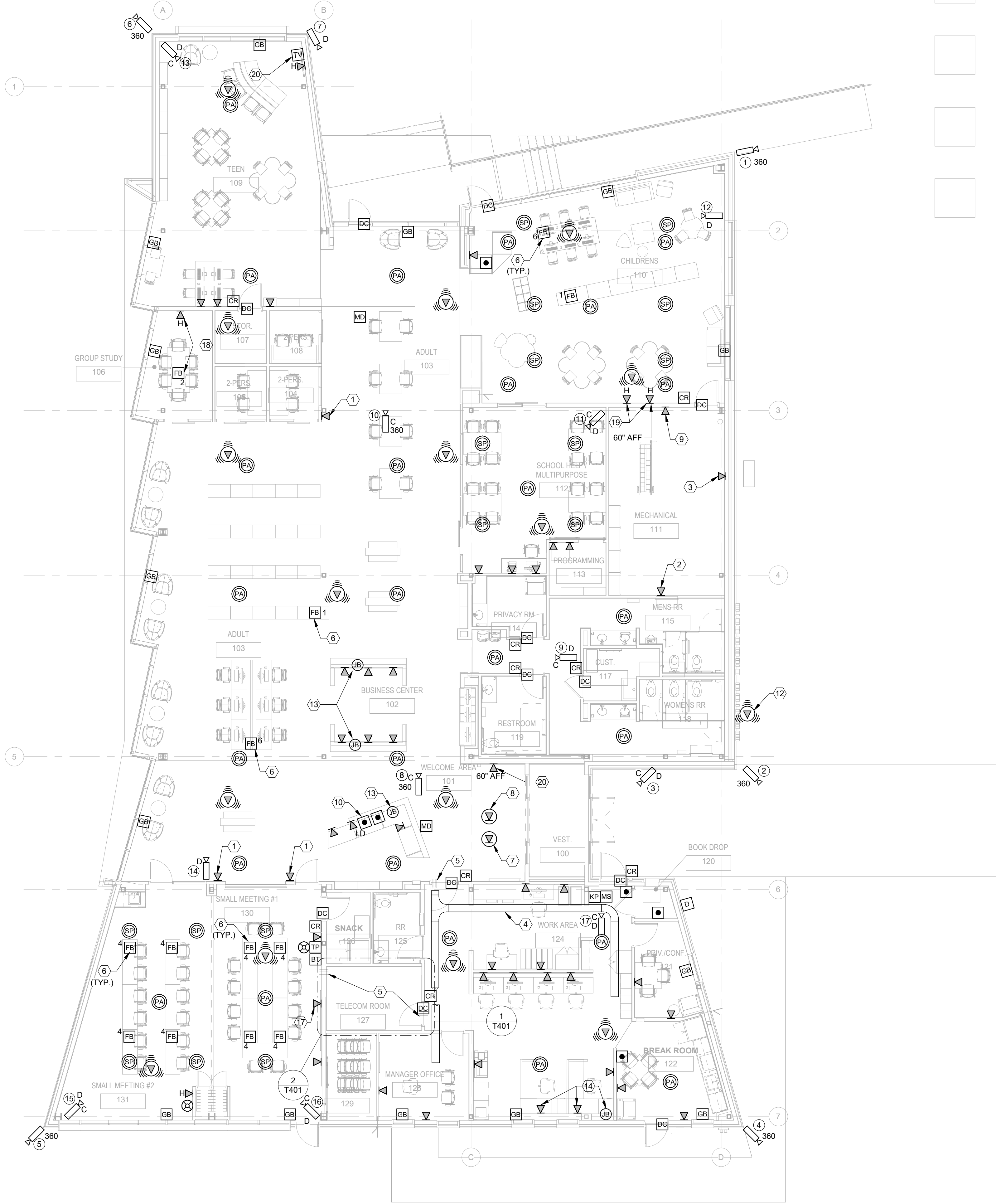
1 FIRST FLOOR PLAN - TELECOMMUNICATIONS 1/8" = 1'-0"
